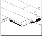
Step 7: Tap end of plank with hammer and tapping block to lock ends of planks together. Remove support bridge and continue with this method until you have completed installing the row.
